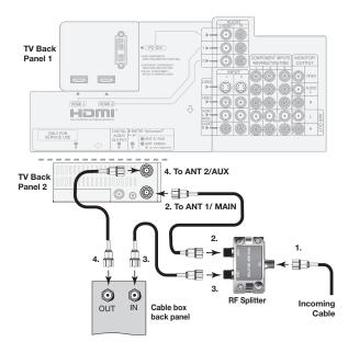
Figure 12. Connecting an older cable box
