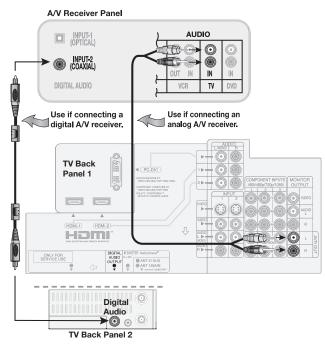
Figure 11. Connecting audio from the TV to an A/V receiver
