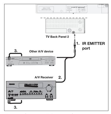
Figure 14. Connecting IR Emitter NetCommand
