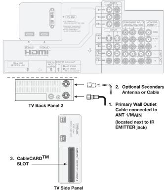
Figure 3. Wall Outlet Cable
