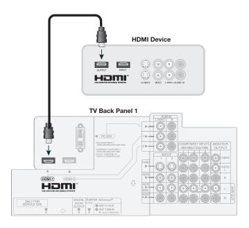
Figure 8. Connecting an HDMI device.
