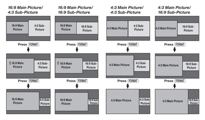
Display choices. Press the FORMAT key repeatedly while in Split Screen mode to view different displays.
