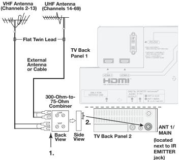
Figure 5. Connecting separate UHF and VHF Antennas
