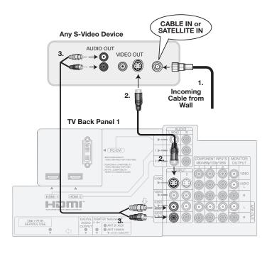
Figure 2. Connecting a device with S-Video
