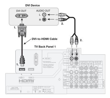
Figure 9. Connecting a DVI device
