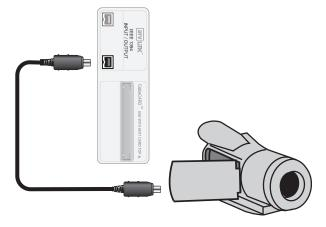
Depending on your camcorder model, you may be able to control it using the TV's remote control by connecting the IEEE 1394 cable. Connect the 1394 cable and try controlling the camcorder, even if you are using analog connections for audio and video.
