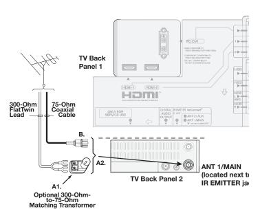
Figure 4. Connecting a Single Antenna
