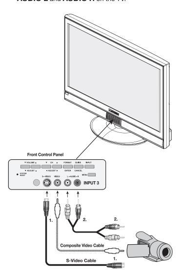
Figure 13. Analog connections for a camcorder
