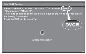
Figure 7. The New 1394 Device screen shows the device name and includes a check box for an associated analog connection.
