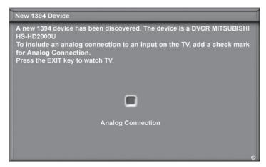
Figure 7. The ClearThought Auto Input sensing screen for IEEE 1394 devices. Place a check in the Analog Connection box if your device has both analog and digital outputs.
