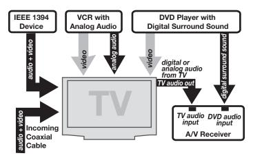
Figure 14. Overview of A/V receiver connections described
