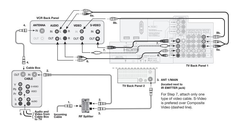
Figure 7. Connecting a VCR to a cable box
