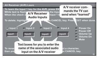
Figure 15. The AV Receiver (AVR) Learn screen lets you set up NetCommand control of your A/V receiver.
